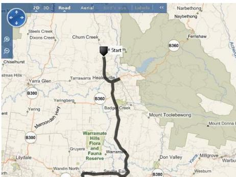
The Mini MT logs its location each 45 Seconds ( adjustable ) If The Mini MT is not being moved it goes to Sleep Mode to save power, but wakes up again on movement or button press.
